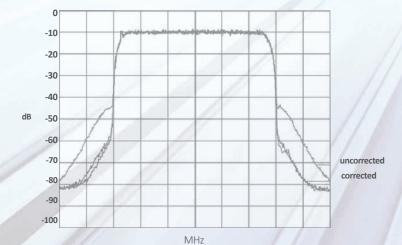
required to meet spectral emission compliance, but the filter itself introduces an undesired distortion. With linear pre-correction, the transmitted signal has optimal modulation performance so less equalization is required at the receiver.
