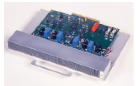
RF Power Amplifier
