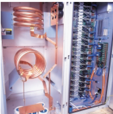
Output Network (left), RF Combiner (right)
