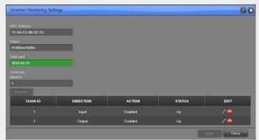
The Monitoring Settings panel shown above allows codec users to configure monitoring for each audio channel. IntraAlert then enables audio stream monitoring and various notifications and/or email alerts. This panel consists of various entries such as **Action**, which if enabled will activate webpage/app notifications and email alerts based on an *alert frequency* chosen by the user.
