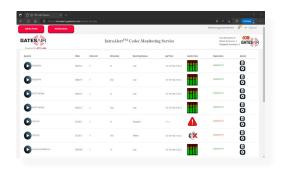
IntraAlert™ is an easy-to-use web and smartphone app-based monitoring solution that allows station owners/operators to monitor multiple codecs from a single interface. It provides real-time health status, uptime, VU meter, and email alerts for each monitored audio channel, making it an indispensable tool for any broadcaster.
